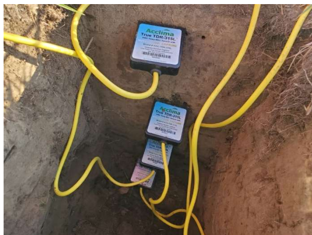
Figure 2.2.1. Installation of Acclima TDR-315 at GPRT1H field location for 6, 18, 30 and 42 cm.
