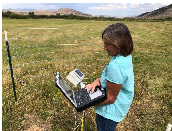
Figure 2.2.2. Field Technician accessing Acclima Solar DataSnap SDI-12 data logger within instrument enclosure protected by cow panels.
